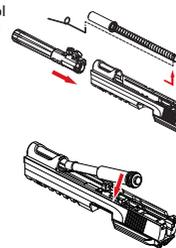
④ Assemble the slide to the receiver from the front and insert the slide stop when the notch is aligned to slide stop's corresponding position. The recoil spring guide set is still contained by now.
