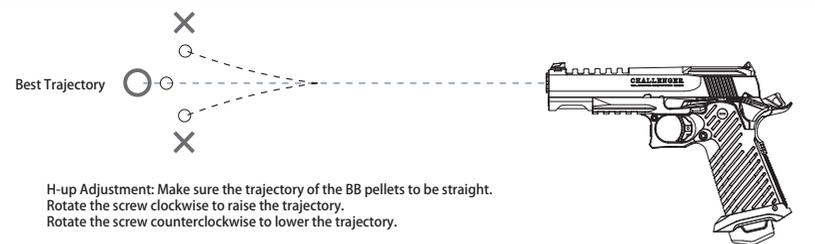
H-up Adjustment: Make sure the trajectory of the BB pellets to be straight.
