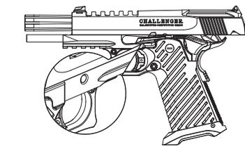
⑤ Press the slide stop button on the right to remove it.
