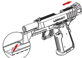
④ Push the Slide backward and align the notch corresponds to the slide stop as shown.
