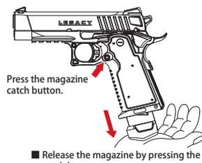
Release the magazine by pressing the magazine catch button.
