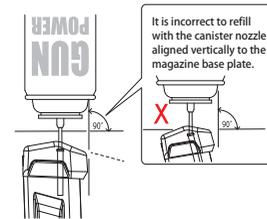
It is incorrect to refill with the canister nozzle aligned vertically to the magazine base plate.
