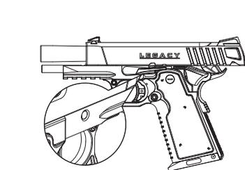
⑤ Press the slide stop button on the right to remove it.
