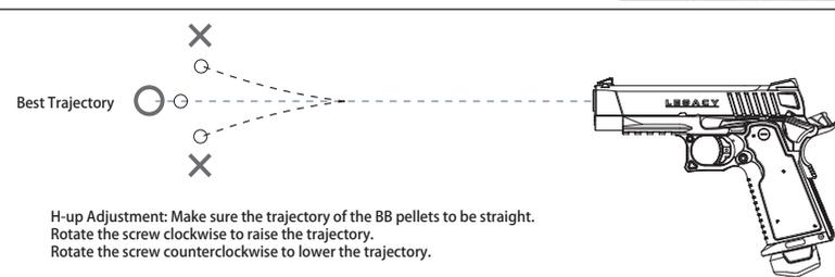
H-up Adjustment: Make sure the trajectory of the BB pellets to be straight.
