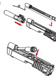
④ Assemble the slide to the receiver from the front and insert the slide stop when the notch is aligned to slide stop's corresponding position. The recoil spring guide set is still contained by now.
